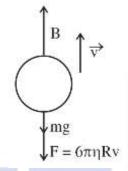
(Because of density of air the value of mg can be neglected)
